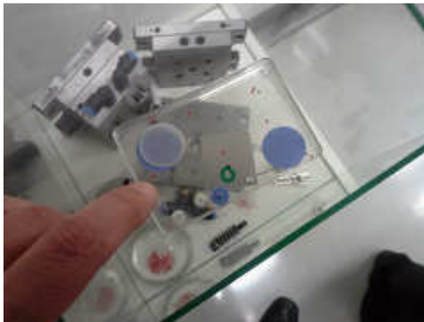
Micro gears (in red) injection molded at the TGI
